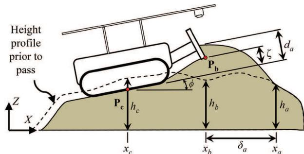
Fig. 2 Illustration of the state variables  $d_a$ ,  $x_b$ ,  $z_b$ ,  $z_c$ ,  $\varphi$ , and  $\zeta$ ; and auxiliary variables  $h_a$ ,  $h_b$ , and  $h_c$  (note that  $P_b = [x_b \ z_b]^T$  and  $P_c = [x_c \ z_c]^T$ )
