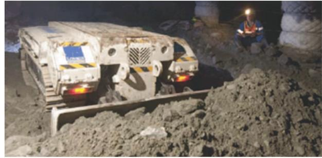
Fig. 1 Teleoperated bulldozer used for underground mining
