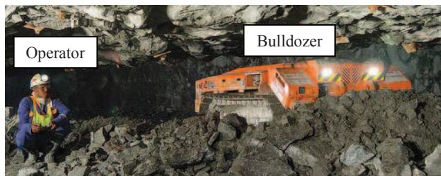
Figure 1: Teleoperated bulldozer used in underground mining.
